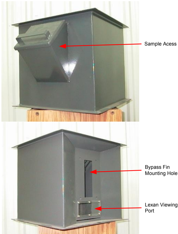
Figure 83 –In Line Chute Example
