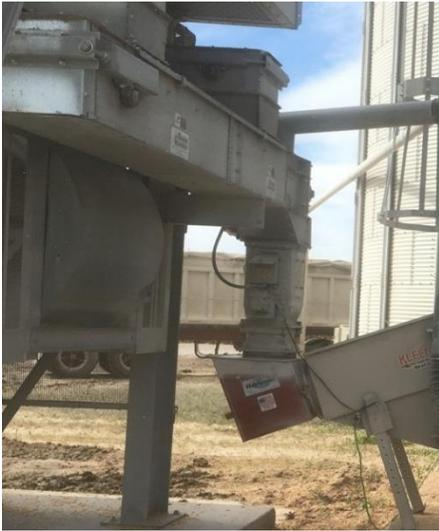
Figure 60 - Inline Chute installation
