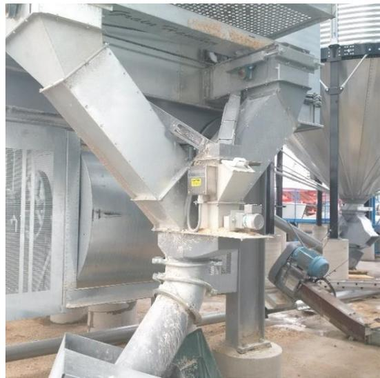
Figure 56 - Example installations of bypass chute with rotary metering
